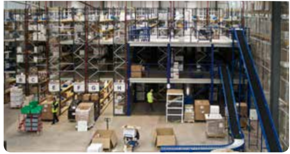
The mezzanine floor integrates with the pallet racking pick tower to create a working area for the conveyors.
