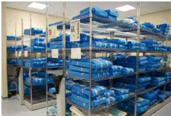
Wire shelving was mounted onto mobile shelving chassises to help create a high density Sterile Store.
