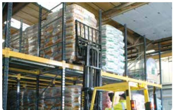
As pallets are picked a safety separator is activated. This holds the accumulated load of several tonnes and allows only one pallet to flow smoothly and securely to the front face.
