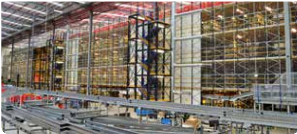
Up to ground plus 4 floor levels are achievable, delivering great space utilisation and flexibility.
