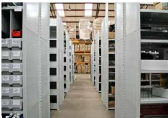
Cross aisles help cut down journey times in picking operations helping to increase efficiency and improve fire escape routes.
